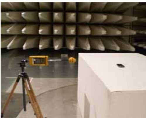
Figure 54 – RF Emission Test of a Mobile Phone
