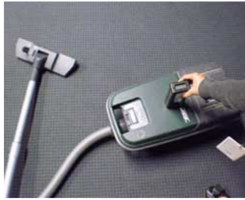
Figure 57 – Magnetic Field Test of a Vacuum Cleaner
