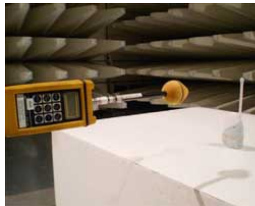
Figure 55 – RF Emission Test of a Baby Monitor
