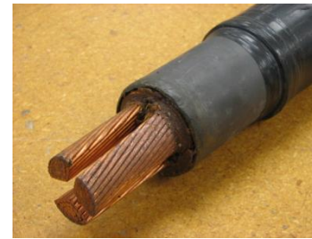
A 3-phase underground cable.
