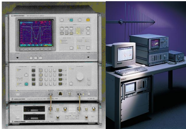
Rhode & Schwarz TS9975 Test Set for 5 MHz to 2.7 GHz.
